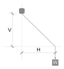
Minor adjustments to a rigging system can have a significant impact to the forces acting on the rigging. For example making a bridle shallower or taking an extra wrap on a sling around a truss to gain a slightly higher trim height. The use of pulleys in a rigging system will also have an effect on the resultant loads. The following table shows typical load factors:
