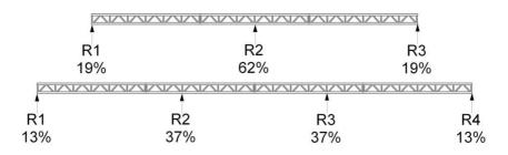
To approximate point loads on these systems the point load can be divided between the two adjacent points as per the equation on page 13. When using the addition of points to provide redundancy then the system has to be tested to the following criteria:
