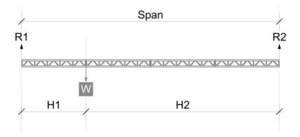
The resultants for a single point load can be calculated as follows:
