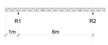
The distribution of load from the cantilever to the hoists on a 2 point pickup can be assessed as per the calculation on page 15 of this guide. In the case of a multi-point pickup, the load would generally all be applied as load to the nearest hoist.
